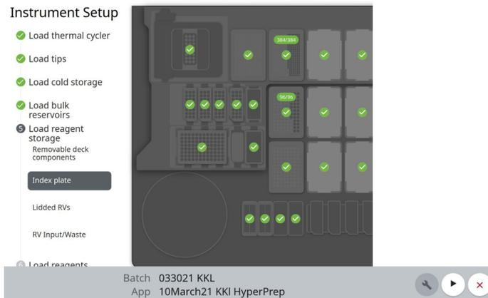
**Figure 5.** Biomek NGenius Dynamic DeckOptix software scans the deck for common setup errors.
