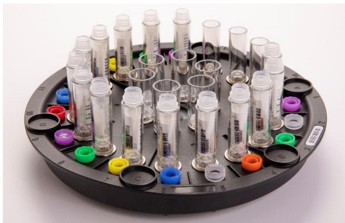
**Figure 4.** Biomek NGenius reagent input carousel can take many of the industry tubes including 0.5 mL, 5 mL.
